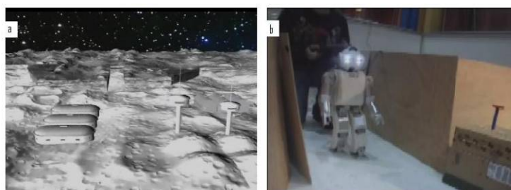
Figure 5 - a) the recreation of lunar scenario. b) HOAP-3 teleoperated through a corridor looking for the ‘antenna’
